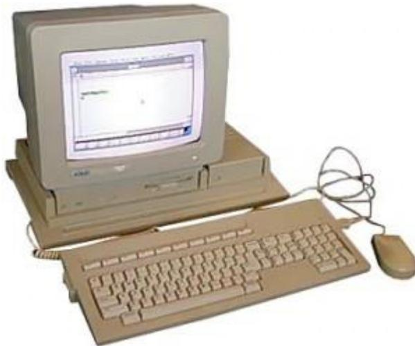
*The Atari Mega STE was Atari Corporation's last ST series personal computer, released in 1991. The MEGA STE was essentially a late-model 680x0-based STE mounted in the case of the otherwise unrelated Atari TT computer, although a number of TT features were also blended in. The resulting machine was a more business-like version of the ST line.*
